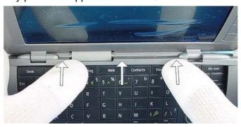
4. Ensure that both snaps on the front side are properly locked.
