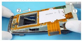
17. The PDA LCD MODULE is attached with an adhesive tape to the C-COVER. Push the LCD MODULE with two fingers slowly and the adhesive peels away.
