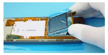
11.Use SRT-6 as a lever to open the A-COVER LOCKING.
