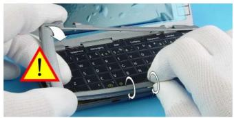
7. Place SRT-6 between the KEYPAD FRAME and the B-COVER and open the first snap carefully.
