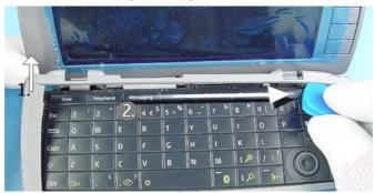
6. Bend the left side of the KEYPAD FRAME carefully and unlock the snaps as shown.
