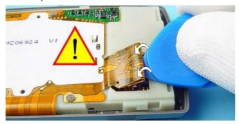
14.Use a slotted screwdriver as a lever to open the clip.
