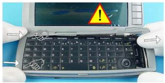
3. Carefully press the upper side of the QUERTY FRAME onto its place.
