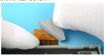
2. Use SRT-6 to remove the remaining adhesive tape.
