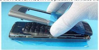
4. Remove the CMT KEYMAT. Note the guide pins when reassembling.
