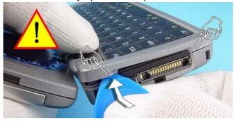
5. Unlock the hooks along the edge of the KEYPAD FRAME as shown.
