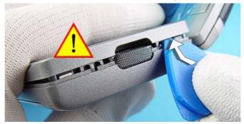
9. Remove the KEYPAD FRAME. Do NOT re-use the KEYPAD FRAME!
