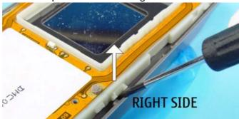
16. Lift out the UI CHASSIS as shown.
