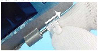
2. Use SRT-6 to push in the A-COVER LOCKING and unlock the A-COVER.
