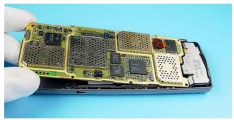
17.Use SRT-6 to push out the CAMERA MODULE from its holder
